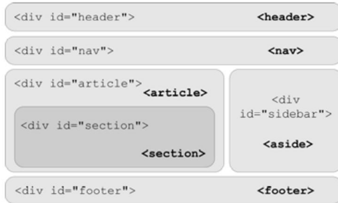
Figure 1. The current (using div elements) and the new approach (using new elements which are presented in bold text) to structuring a web page
