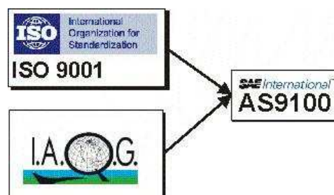
Figure 1: AS9100 – ISO 9001 and additional Aerospace requirements identified by International Aerospace Quality Group (I.A.Q.G.)
